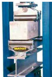
Flexure on concrete
