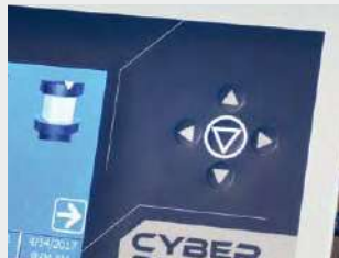
Traditional directional key pad with 5 arrow-keys for standard use or when wearing gloves
