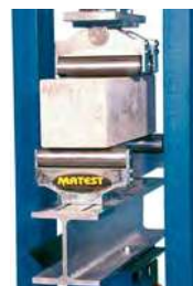
Flexure on concrete
