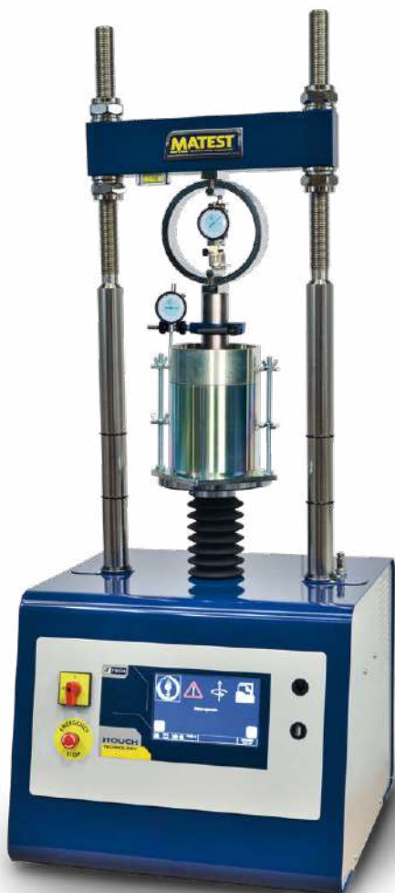
S212M with accessories for CBR test
