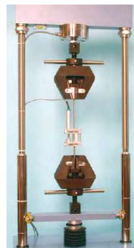
S205-05N + accessories for tensile test
