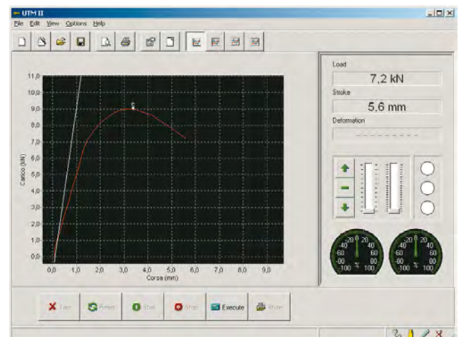
B043-01N: Load/deformation "x-y" graphic example
