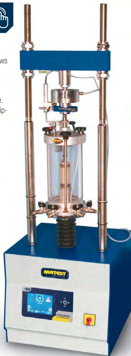
S301N with data acquisition
