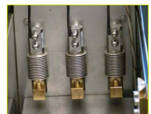
Detail: 3 load cells 500 N
