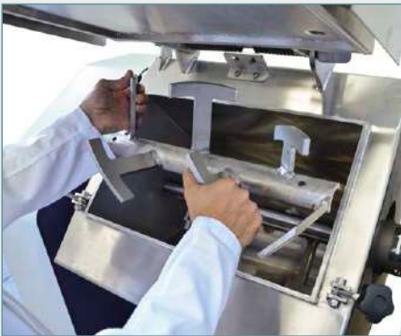
B026-05N Detail of the detachable mixing shaft
