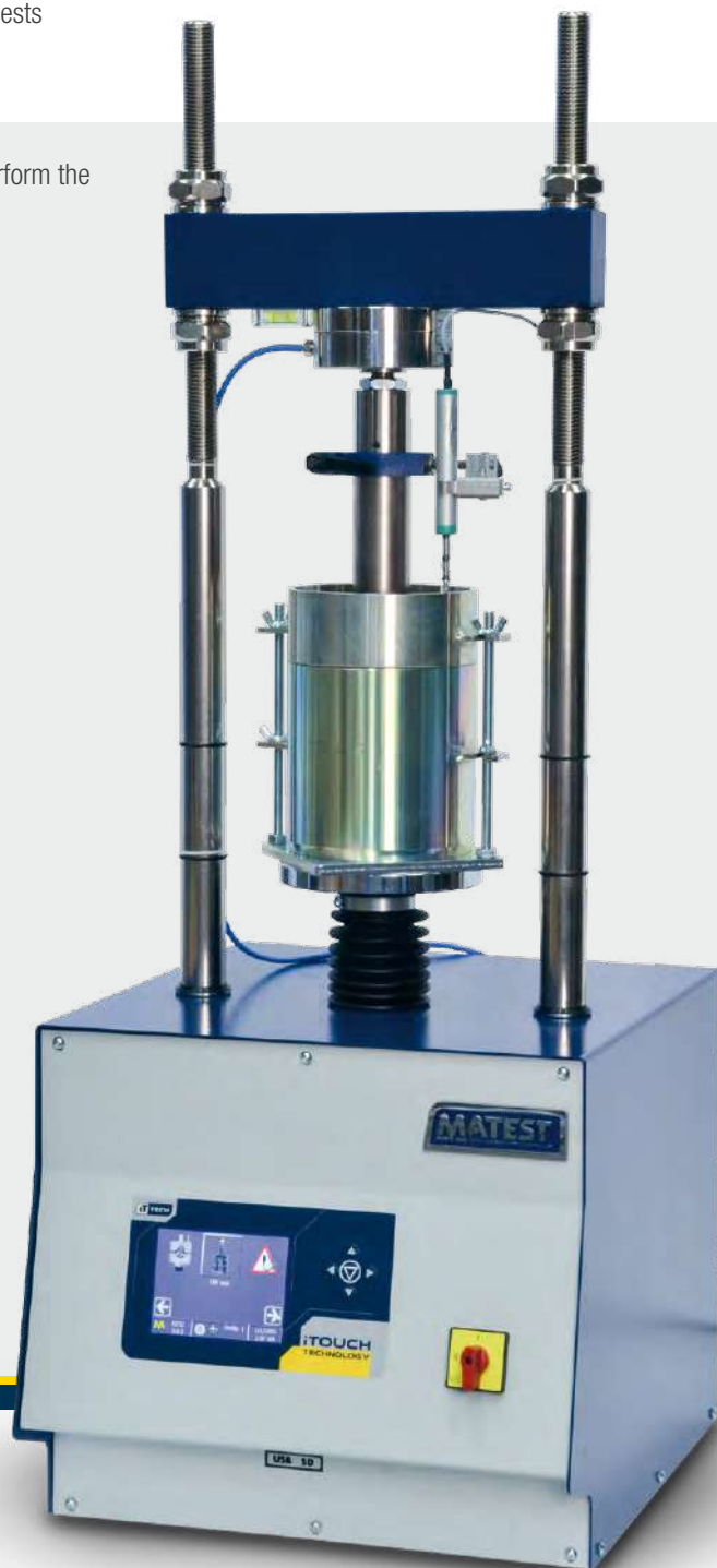
S215A with CBR mould
