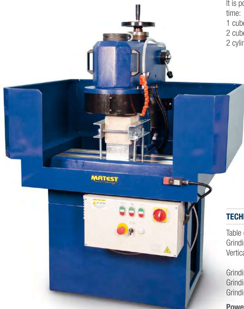
C299 with C300-06N holding one 150 mm cube
