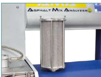
Integrated balance for automatic weight record
