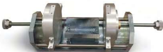
B282-08 TSRST specimen gluing jig (needed accessory)
