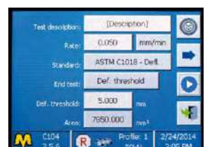
C109-15N Set up of deflection
