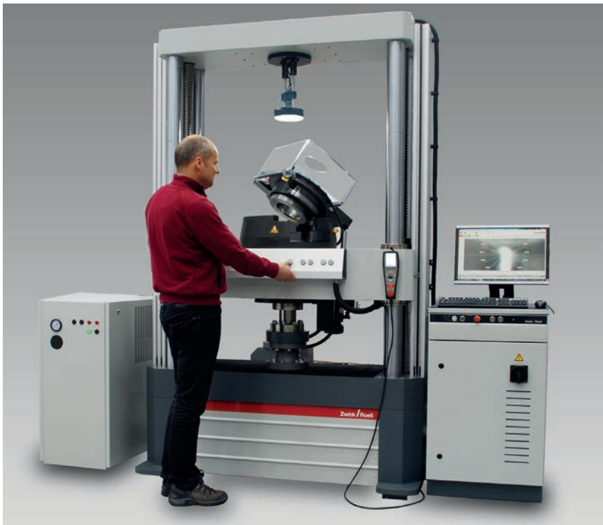
Fig. 1: Sheet metal testing machine with videoXtens
