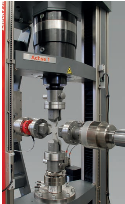
Fig. 2: Biaxial testing machine with superimposed torsion
