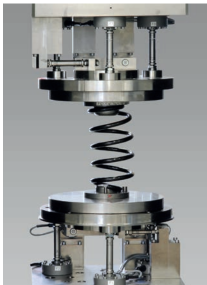
Fig. 1: Multi-channel tests on suspension springs
