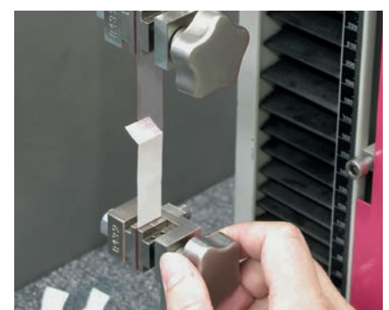
Fig. 7: Peel tests on adhesive strips
