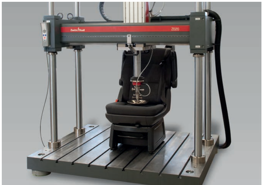
Fig. 2: Flexible test bench for characterizing seats
