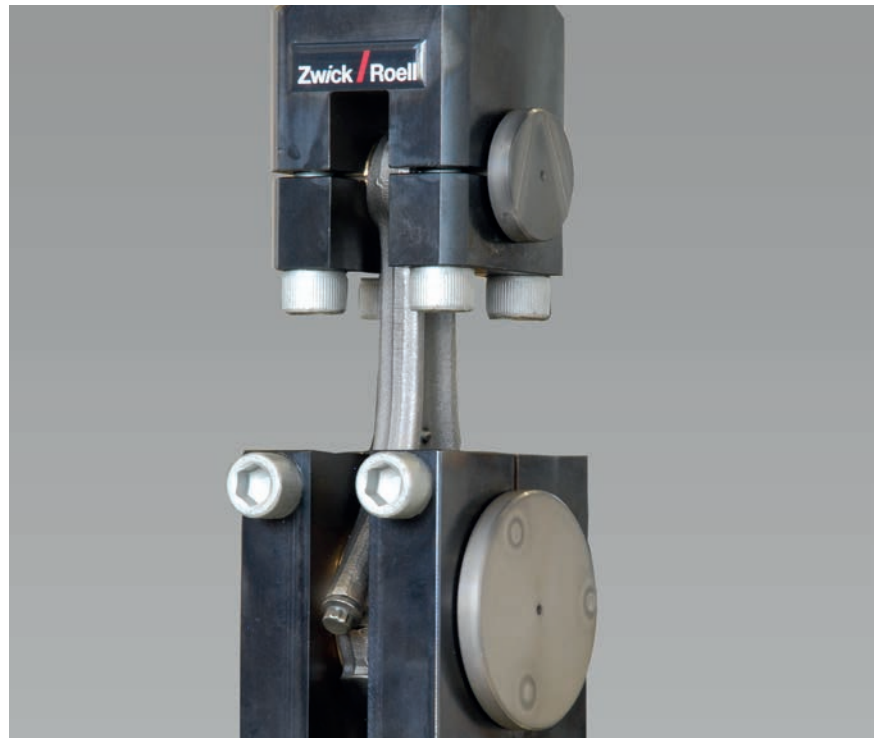
Fig. 1: Fatigue tests on connecting rods
