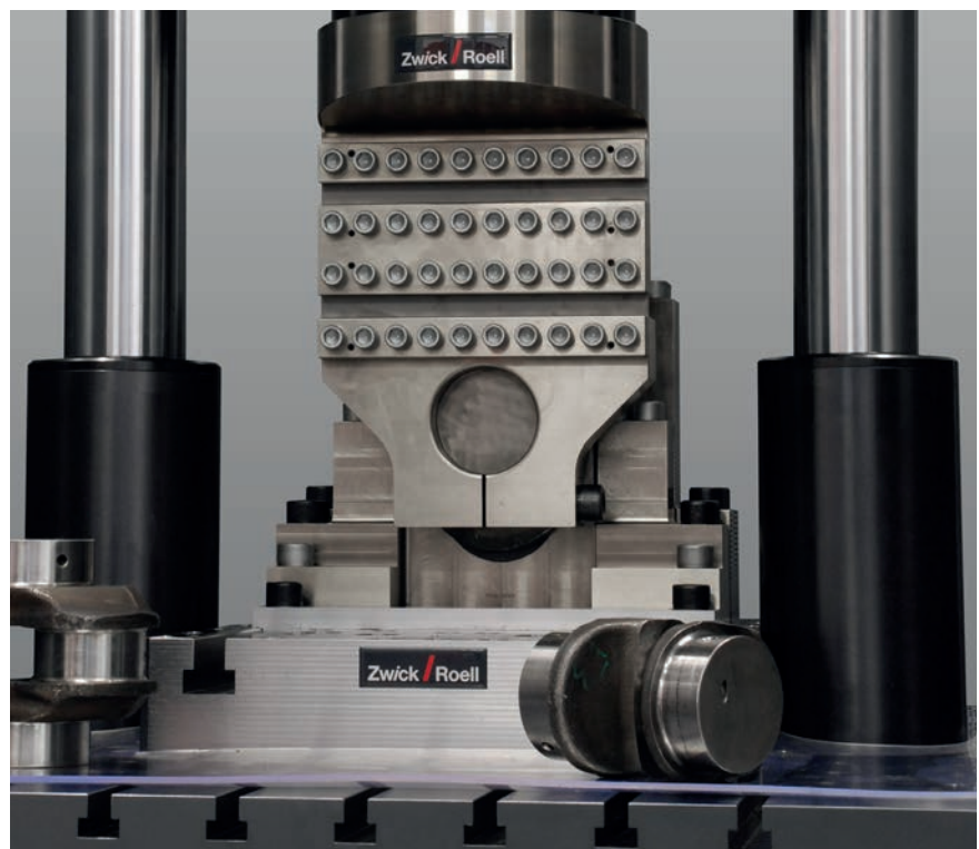
Fig. 2: Crankshaft segment under dynamic loading in a Vibrophore
