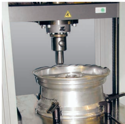
Fig. 3: Testing axial deformations of the rim flange
