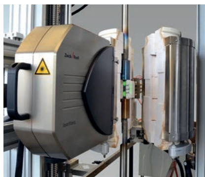
Fig. 4: High-temperature furnaces can also be retrofitted
