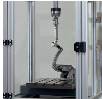
Fig. 4: Fatigue testing of an emergency brake lever
