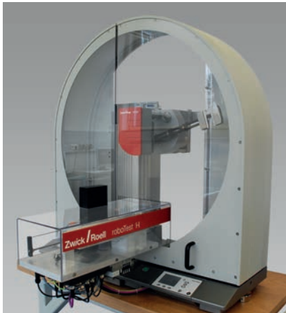
Fig. 1: HIT50 P Pendulum impact tester with automatic specimen feeding
