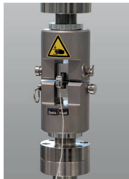
Fig. 2: Determination of the fracture toughness K_{Ic}
