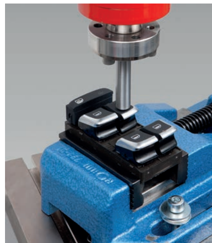
Fig. 2: Function tests on a window lifting switch element
