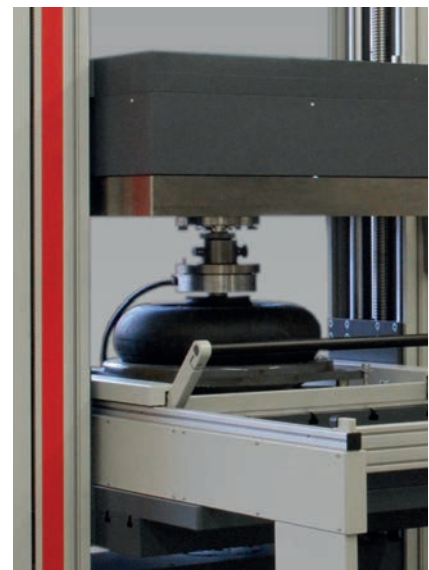
Fig. 2: Testing of pneumatic springs
